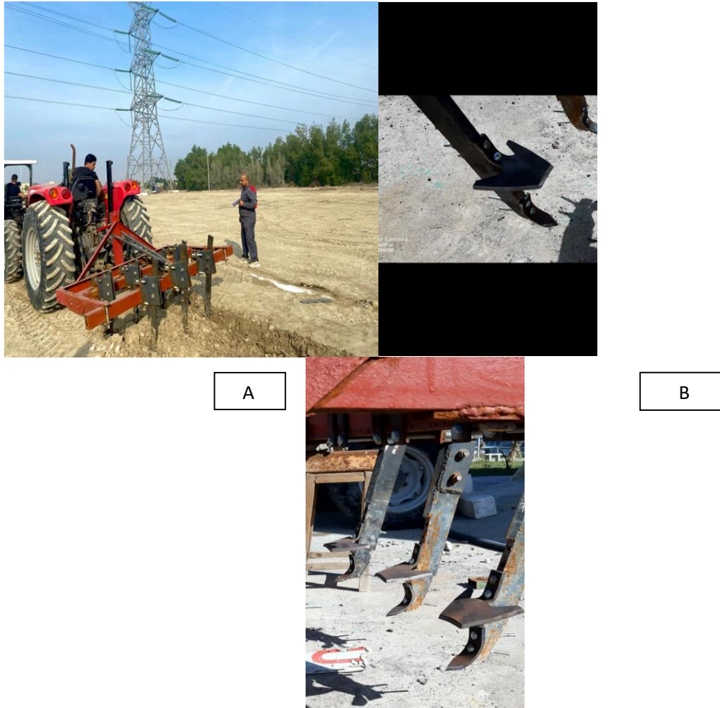
Figure No. (2) A View showing the weapons used in the plough B A view showing the developed drill plough during the experiments.
